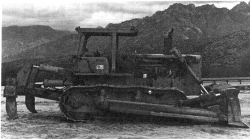
Bulldozer. Note the smoke stack (exhaust pipe).
