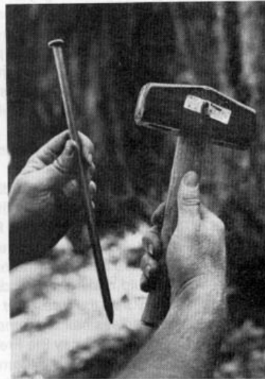
A bridge timber spike and single jack hammer for use with very large trees. Smaller spikes are fine for general use and can be driven in with a heavy standard hammer.
